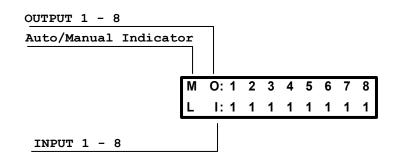
If no audio is being fed to the unit on any channel the numbers in the lower half of the display will be inverted indicating no audio present. After 5 seconds of audio application on a given channel above threshold the respective lower channel indicator will become un-inverted indicating audio present above the on the channel.
