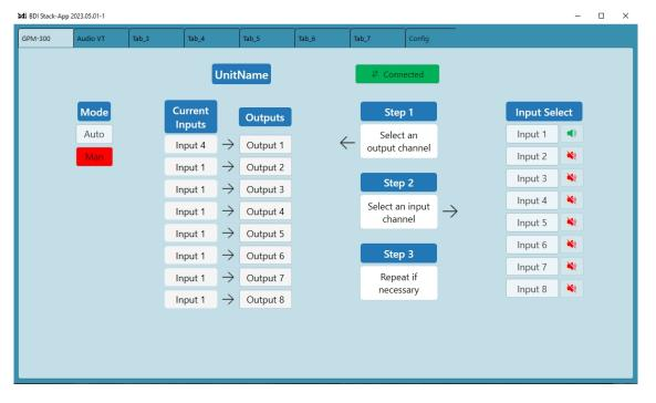
Follow the on screen instructions for channel selection. The speaker ICON next to each input indicates audio presence. When green audio is present on the channel. When red audio is absent on that channel. The GPM-300 series audio switchers can be controlled and monitored via SNMP v2. You can download the MIB for this product at the link below:
